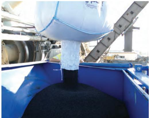
At the request of the Virginia Department of Transportation Research Council (VTRC), Boxley partnered with Iterchimica to test the viability of Gipave, an innovative asphalt that utilizes unrecyclable plastics in the mix.
